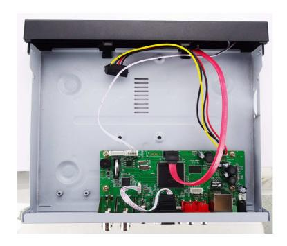
Step 3) Connect SATA & Power wire to Hard Disk and put it on the rack mount.
